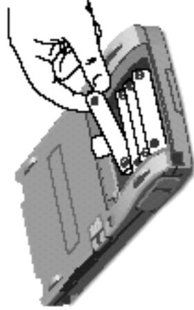
The tab that you pull to remove the batteries should stick out as shown above the topmost battery.
