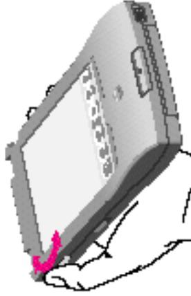
**Optional:** If you purchased the Newton power adapter, you can connect it to your MessagePad and plug it in to conserve battery power. The power adapter plugs into the port beneath the rubber flap marked with the
