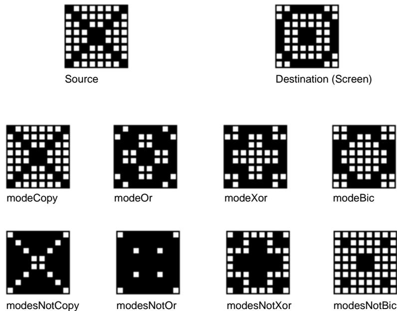
In Figure 3-8, the Source item represents something being drawn on the screen. The Destination item represents the existing bits on the screen. The eight patterns below these two represent the results for each of the standard transfer modes.
