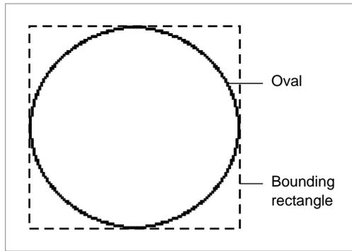
An **arc** is a portion of the circumference of an oval bounded by a pair of radii joining at the oval's center; a **wedge** includes part of the oval's interior. Arcs and wedges are defined by the bounding rectangle that encloses the oval, along with a pair of angles marking the positions of the bounding radii, as shown in Figure 13-4.
